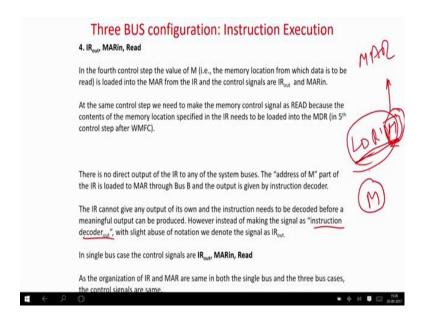
So, the memory data register we are connecting to both A and B. So, in this case you have to explicitly specify that where you have to go connect basically because we have to go to instruction register and instruction register is basically connected to B. So, in this case we are saying  $MDR_{outB}$ .
