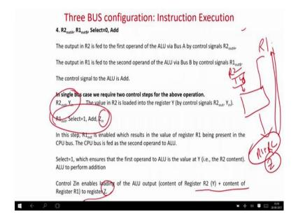
So, what we have to do? We have to take  $R_{2out}$  and  $Y_{in}$ . So, what was that? We have to take the value of  $R_2$  and store in a temporary register that is actually equal to Y if you remember it is a temporary register Y we are now having the value of  $R_2$  over here one step is gone.
